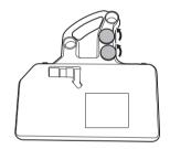
4 Secure the two caps onto the two holes by turning them clockwise.
